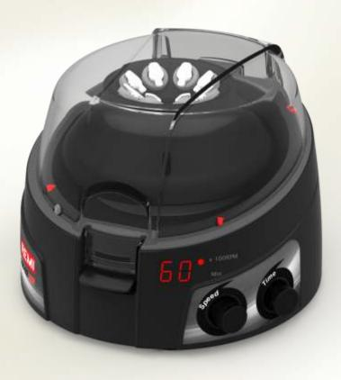
Powerful and easy-to-use RM 02 Plus mini centrifuges are small enough so that each workstation can be equipped with a personal centrifuge.
