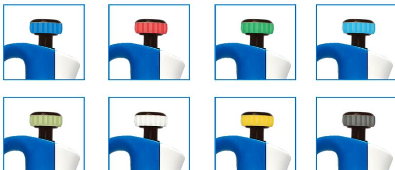
Colour-coding for different capacities facilitates easy identification during daily laboratory routine
