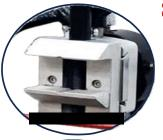
Holds the paraffin block in place, typically, the block moves up and down with each revolution while the blade is stationary. Block holder allow the usersto manipulate the block face in various direction to bring the tissue in alignment with the blade.
