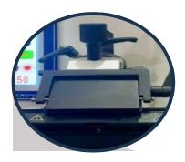
Blade holder slides sideways in both directions allowing the use of the entire cutting edge. It accepts either low or high-profile blades. Guard is provided for the user protection. Stage is coated for easy flow of section.
