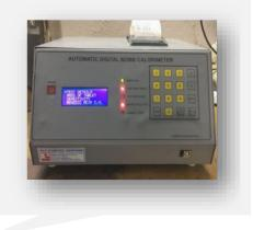
SAMPLE TEST MAX.TEMPERATURE 00.74 C WATEREQUIVALENT 2467 MASS OF TABLET 0.300 GM CV 5956.46 CAL/GM 09:05 22/09/17 REPORT NATER EQUIVALENT TEST MAX.TEMPERATURE 02.44 C SENZOIC ACID CV 6320 MASS OF TABLET 0.930 GM NATER EQUIVALENT 2517 14:35 28/07/17 CALIBRATED ON:- 5/1/17
