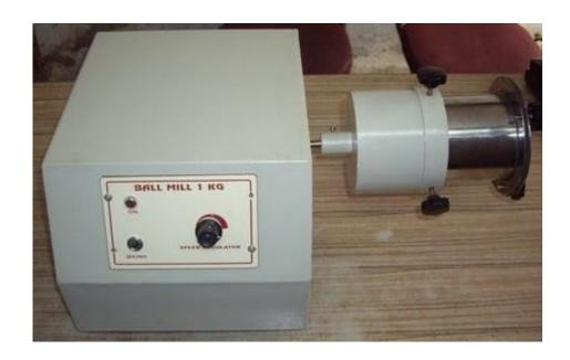
A drum is made of welded steel having an inside diameter of 300 mm x 300 mm long. Supported on heavy duty ball bearings. An air and watertight cover is provided to close the 100 mm. Wide opening along with entire length of the drum. A reduction gear driven by a motor rotates the mill at 28 - 30 rpm. Supplied complete with twelve 19 mm. Diameter hardened steel balls and an automatic revolution counter. Operation on 1 H.P. motor, 220 / 230 V, 50 Hz. Single Phase Main AC.
