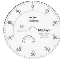
Graduation: 0.01 mm, Measuring range: 5 mm Waterproof
