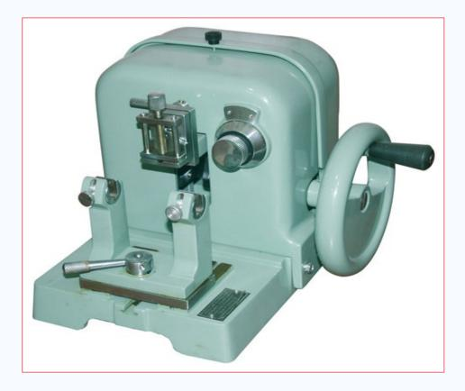
MICROTOME AT GLANCE CONVENIENTLY LOCATED FEED INDICATOR ACCURATE SPECIMEN ADVANCE CONVENIENT SPECIMEN HOLDER SAFETY DEVICE SMOOTH DRIVE WHEEL WITH LOCKING STURDY, RIGID CONSTRUCTION FOR SHAKE PROOF CONSTRUCTION MINIMAL MAINTENANCE PROTECTIVE COVER FOR EASY CLEANING ACCEPT ATTACHMENTS FOR DISPOSABLE BLADES
